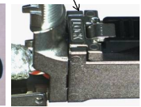
Figure 11b Close Locking latch
