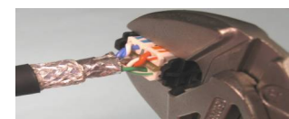
Figure 8 Crimp load bar & wires onto circuit board
