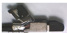
align shields under clamp
