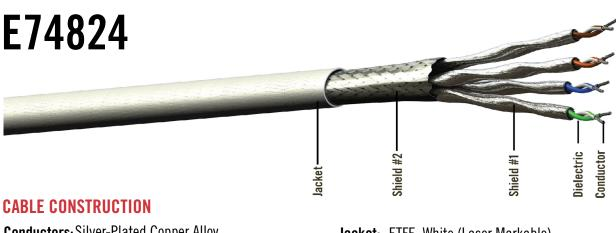
Conductors: Silver-Plated Copper Alloy Dielectric: FEP Shield #1: Aluminum/Polyester Foil (Each Pair) Shield #2 Silver-Plated Copper Braid Jacket: ETFE, White (Laser Markable)
